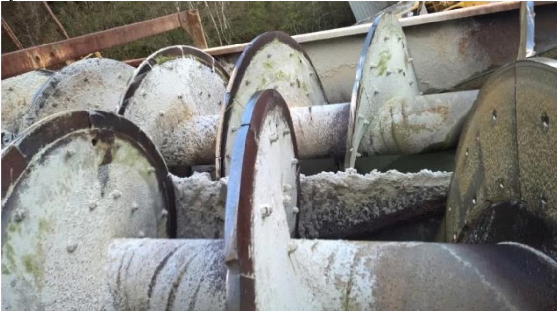
An Archimedes Screw used to lift the sand and water slurry.
